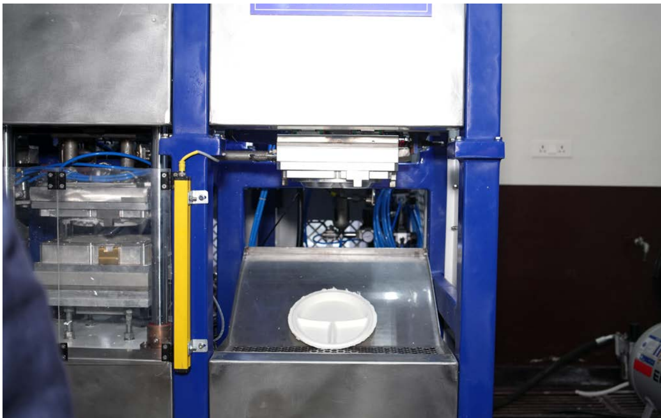
Developed Automated Laboratory Molding Machine with Barrier Coating
