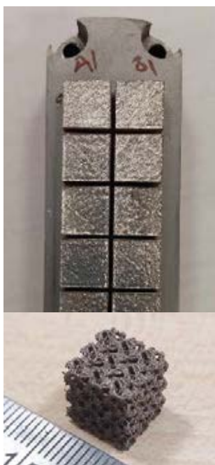
AM coupons made by Powder Bed Fusion (PBF)
