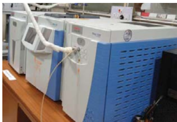
Online high-pressure and high temperature autoclave reactor integrated with GC at IIT (ISM) Dhanbad
