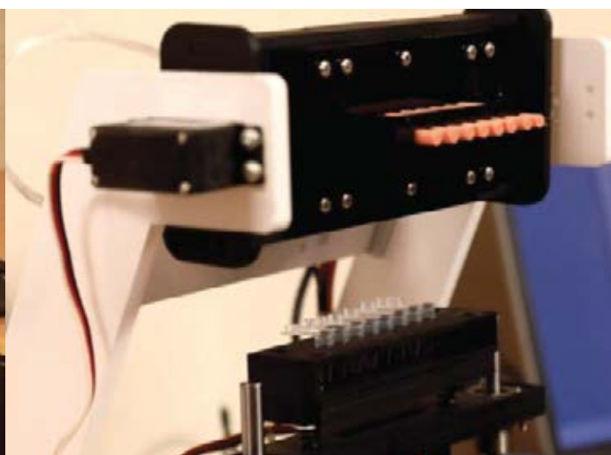
Fabricated 8 channel Array Biosensor Prototype before and after loading the fiber probe cartridges
