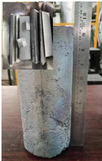
Fe-Mn based alloy ingot made by Vacuum Induction Melting (VIM)
