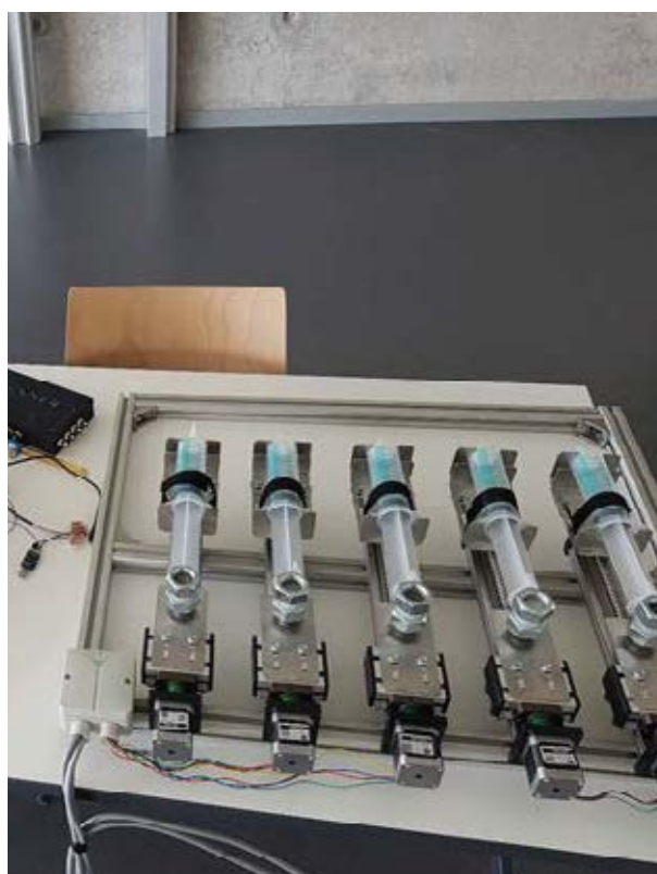
Prototype of the Fertigation Unit with Controller and user interface (Left), sensor array (middle) and injection unit (right)
