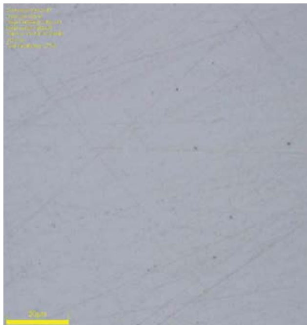
Optical micrographs of the coupon shows defect free
