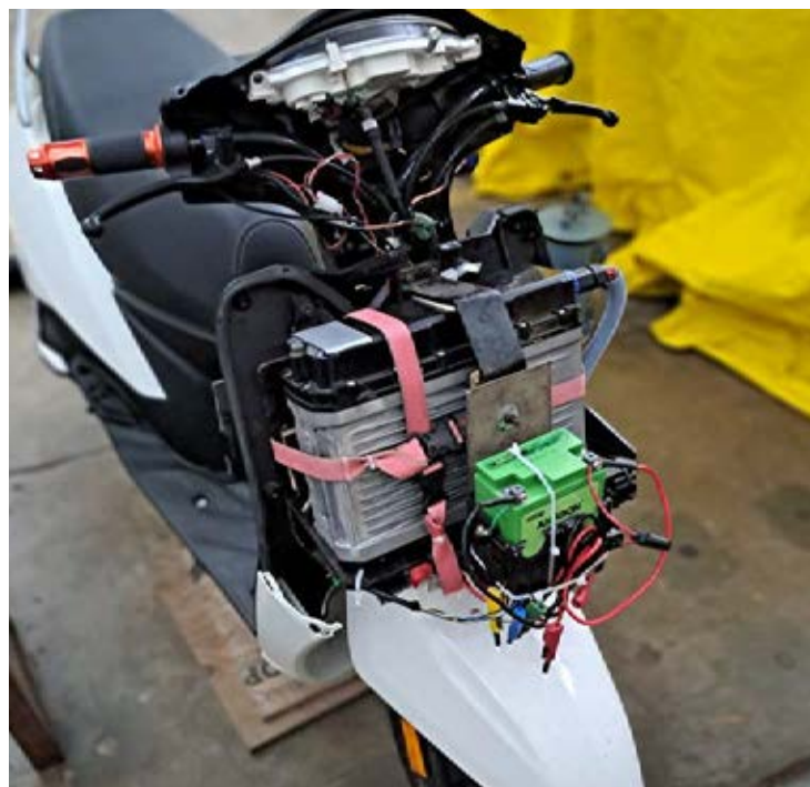
TVS Jupiter two-wheeler with Hybrid Electric Drive
