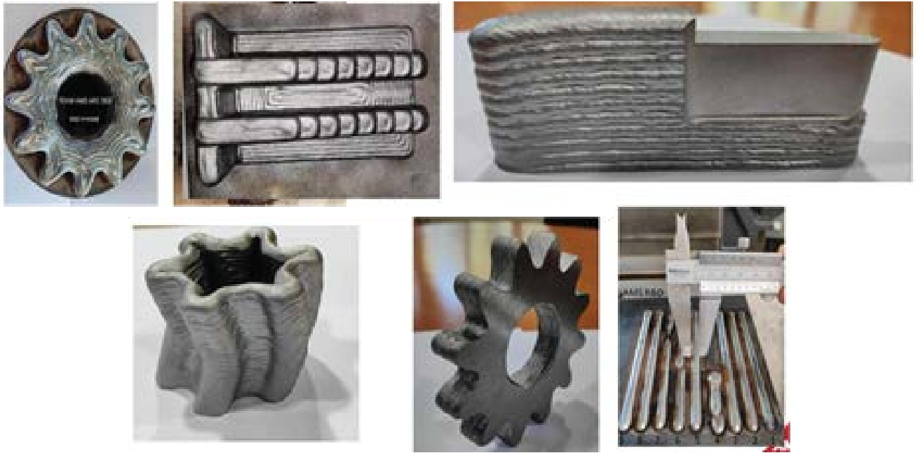
Various 3D printed parts using the Arc Welding technology
