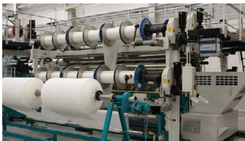
Wrap knitting machine that produces textile substrate at ETF
